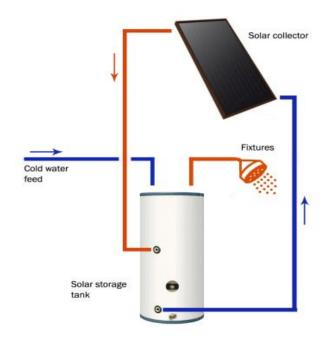
Schematic of a typical solar water heating system
