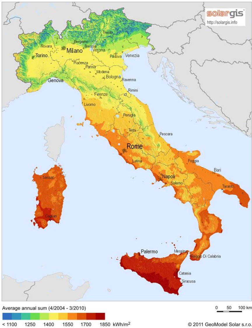
Figure 200: Italy Solar Resources (Horizontal Radiance)
